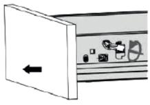
2.Release the Drawer from the slide, pull the Drawer out
