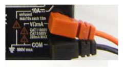
To test that the heating mats are in good working order, firstly you must insert the testing probes into the meter in the ports as illustrated.
