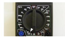
Then set the meter to 2000 In the green (ohms) section.
