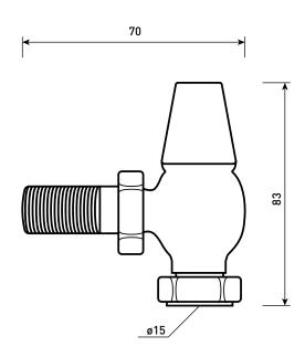
The valves are not bi-directional and should be fitted to the flow side.
