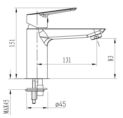
Information: Finishes: 0.2Bar(L/min) 0.5Bar(L/min) 1Bar(L/min) 2Bar(L/min) 3Bar(L/min) 3.7 8.8 12.8 15.8 6.1 Chrome
