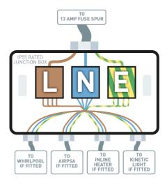
ELECTRICAL CONNECTION - THIS SHOULD BE CARRIED OUT BY A QUALIFIED ELECTRICIAN
