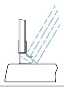
It is important to remember that water will find it's way naturally. This is a physical law that we cannot change. Our frameless bath screens are designed as a deflector for water to try and reduce the chance of water escaping from the showering area over a bath during normal showering conditions.
