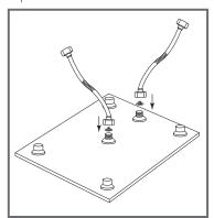
1. Screw the Water Hoses to the Shower Head making sure to insert the Gauze Filters (x2).
