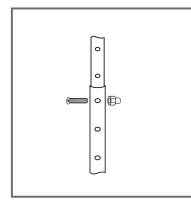
5. Offer the Shower Head up to the ceiling, keeping level. Set to your desired height and join the Support Legs together using the Round Headed Nuts/Bolts (x4).
