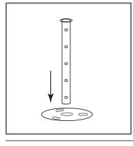
3. Insert the Support Legs (Top) (x4) through the Circular Ceiling Mounts (x4) ensuring that the shiny side faces downwards.
