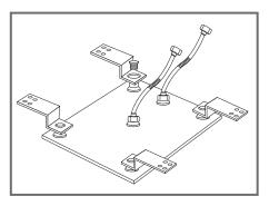
3. Alternatively, attach the Metal Brackets (x4) to the Shower Head upside down to give more height.
