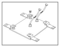
2. Attach the Metal Brackets (x4) to the Shower Head using the threaded Caps (x4).
