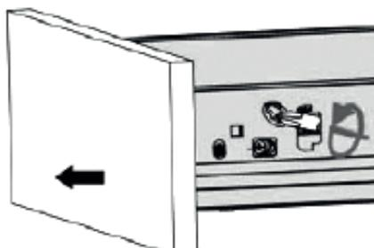
2. Release the Drawer from the slide, pull the Drawer out
