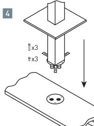
• Hold the main unit in position above the brass boss to connect the inlet pipes
