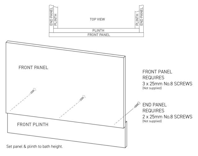
Screw panel onto plinth from behind - DO NOT screw all the way through as screws will protrude through the front.
