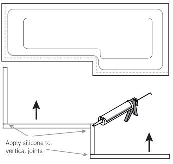
Apply silicone between the **underside** of the bath and the **top** of the bath panel
