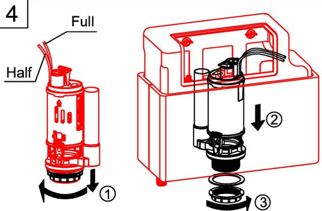
4 As per above picture①:disassemble the lock nut and plastic washer,install the flush valve through out the tank hole(Picture②),make sure it doesn't touch the tank or fill valve.Assemble the washer and lock nut and tighten it, Picture③.
