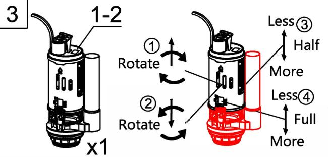
3 You can take out the flush valve body by rotating the flush valve 180° and assemble in same way(Picture ①.②).Adjust half flush: Lift the half flush cup up and down to adjust the flush water less and more(Picture③). Turn the full flush clip up and down to adjust the flush water less or more(Picture④).
