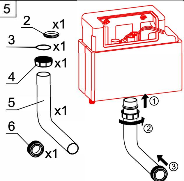
5 As per above picture①:Insert the outlet pipe to the outlet hole of flush valve,(Picture②)Keep flush valve and outlet pipe stand straight and screw the nut as tight as possible.
