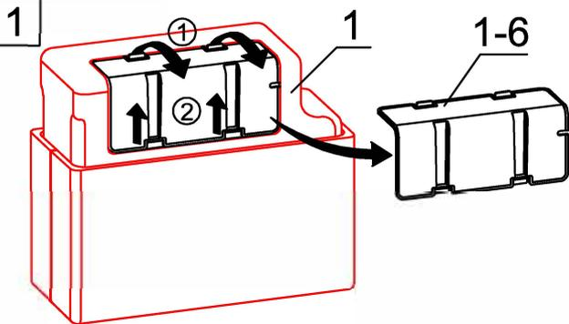
1 Disassemble: As picture①: Pull out two flaps of L cover on top of tank body first. As picture②: Pull up two flaps of L cover on front of tank body to take it out.
