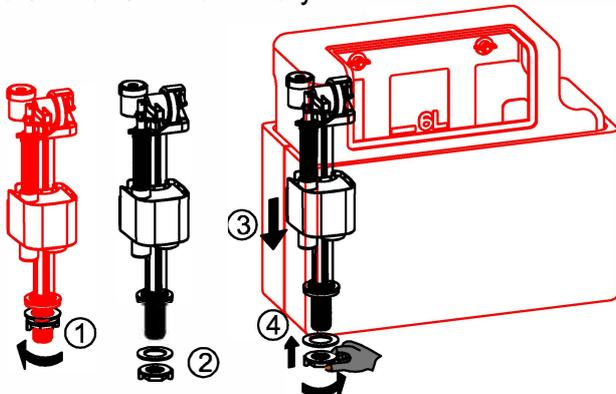
As per above picture①:disassemble the lock nut and plastic washer.Install the fill valve through out the tank hole(Picture③),make sure the fill valve is vertical and doesn't touch the tank. Assemble the washer and lock nut,and tighten it. Attention: Make sure the bowl nut is tightened.
